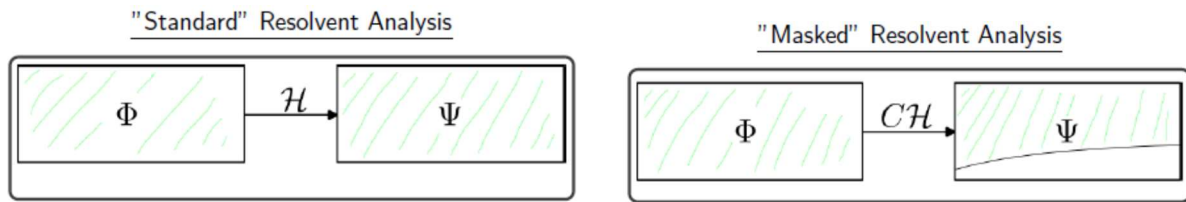
Figure 1: Local and biglobal resolvent analyses, showing masking for the biglobal case in which response is restricted to the freestream.
