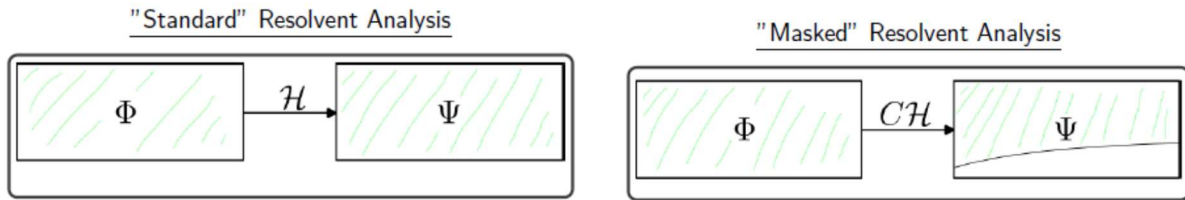
Figure 1: Local and biglobal resolvent analyses, showing masking for the biglobal case in which response is restricted to the freestream.
