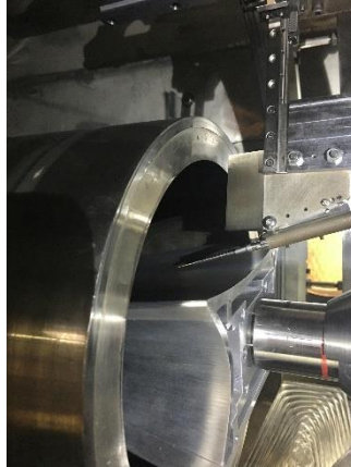
Figure 3-28. Hot-wire located above the surface of BOLT in the M6QT.
