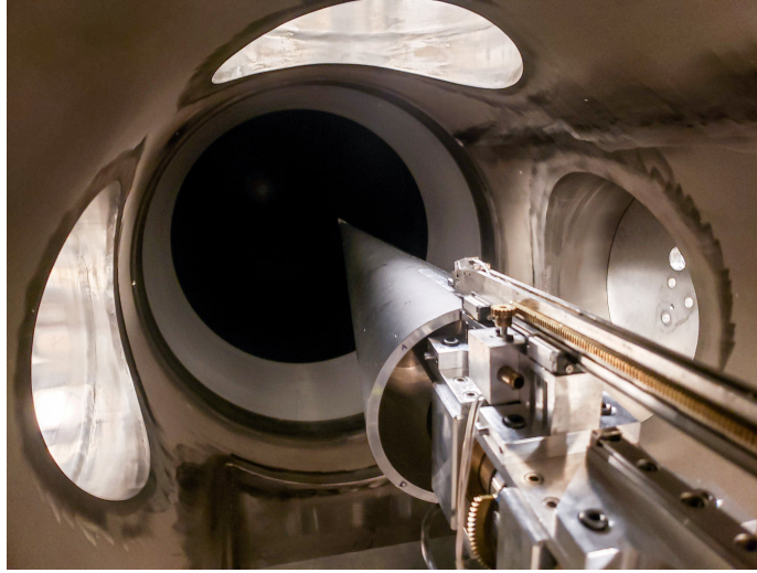
Figure 23: Photograph of cone model in the Air Force Academy Mach 6 Ludwig tube test section.
