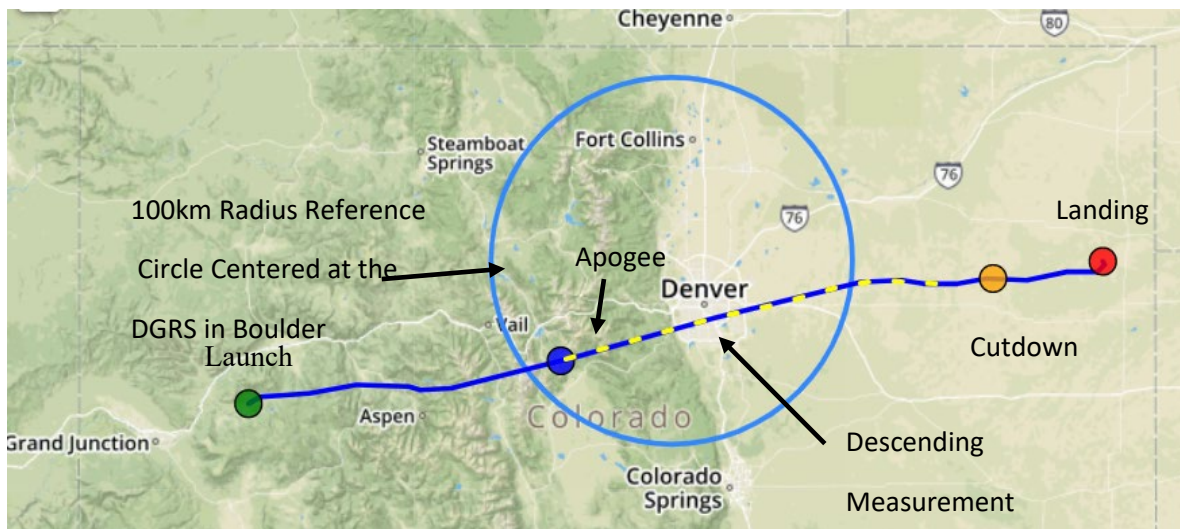
Figure 15 HYFLITS Balloon Trajectory Simulator (BTS) showing ground track for an upstream launch in western Colorado, placing the descending measurements over the continental divide where the largest mountain wave activity is expected. Data is collected by the DGRS station at the center of the large circle.
