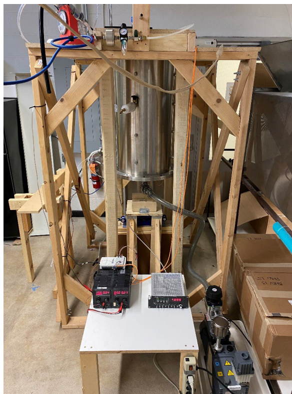
Figure 48 The thermal-vacuum calibration chamber mounted to its support structure. The image on the left shows the aerosol generation system on top of the chamber. The image on the right shows the pumping system on the bottom right of the image.
