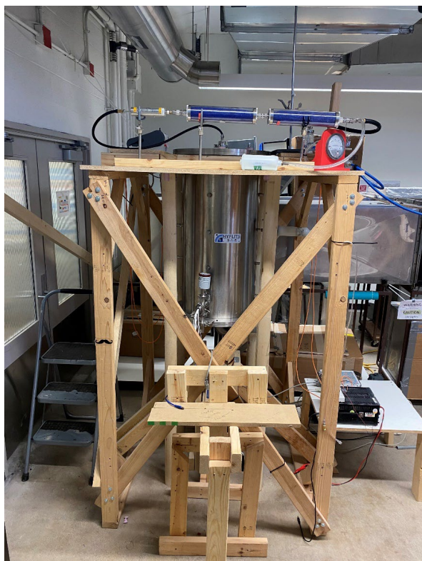
Figure 48 The thermal-vacuum calibration chamber mounted to its support structure. The image on the left shows the aerosol generation system on top of the chamber. The image on the right shows the pumping system on the bottom right of the image.
