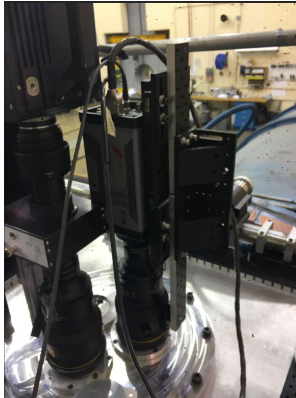
Figure 5: KTV Equipment in AEDC Tunnel 9 Lab. Camera mounted on top of the test section.
