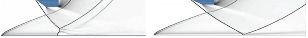
Figure 17: Numerical pseudo-schlieren snapshots for shock generator rotation angles of 0 (left) and 10 (right) degrees.
