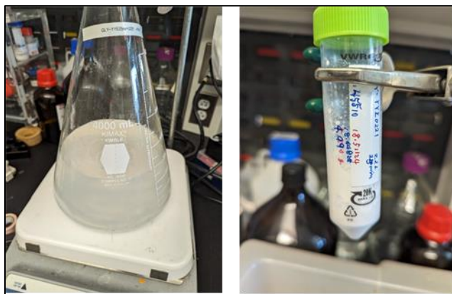
Figure 18. 2 liter aqueous solution amino acid (glycine) mediated synthesis of sodium yttrium fluoride yield 5 grams product, which contains about 2.4 gram REE elements.
