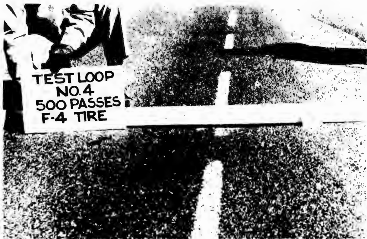
Figure 17. Porous Asphalt Cold Mix After 500 Passes with C-130 and 500 Passes with F-4
