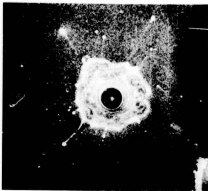
Fig. 4-7 SEM micrograph of SQBD on (100) p-type substrate with Al(-). d_o = 2500\text{\AA} , V_b \sim 185\text{V} , T = 100^\circ\text{K} X2,000
