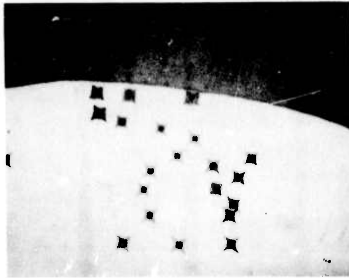
Fig. 5-6 Optical micrograph of anisotropic SQBD's on (100) p-type substrate with Al(+). d_o = 4000\text{\AA} , V_b from 200V to 280V, T = 300^\circ\text{K} X120
