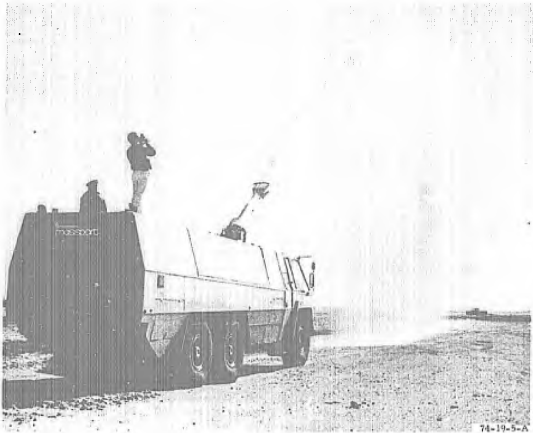
A. PROTEIN FOAM BEING DISCHARGED AT 1800 GAL/MIN OVER THE STEEL GRID CONFIGURATION
