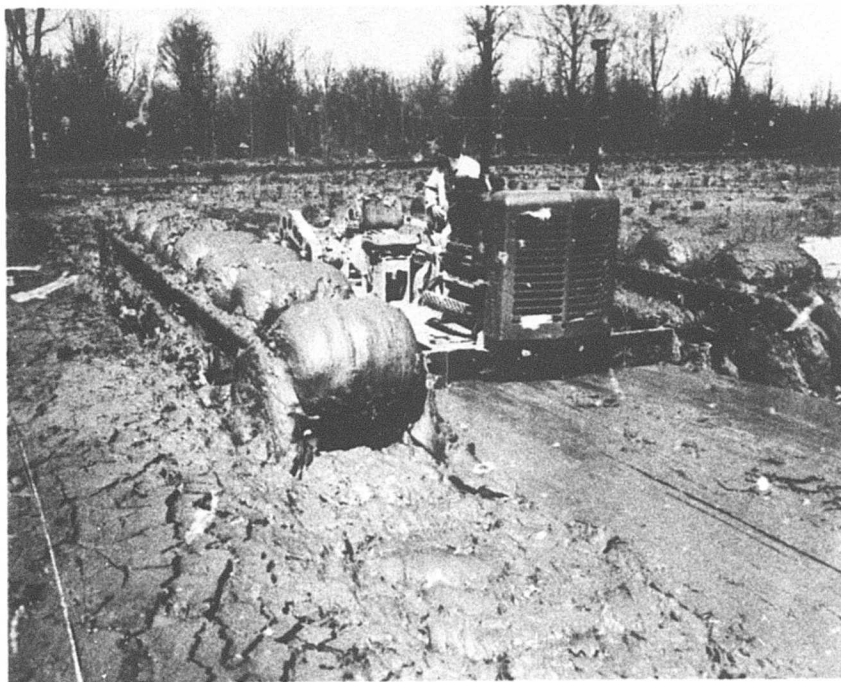
Fig. 18. Airoll on tenth pass (in reverse) in soft sandy clay (test 14, table 1). Note the adhesion of soil to the Airoll's running gear
