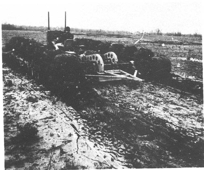
Fig. 16. Airoll rut pattern after 25 passes in soft sandy clay (test 11, table 1). Track slip has sheared the ridges shown in fig. 15
