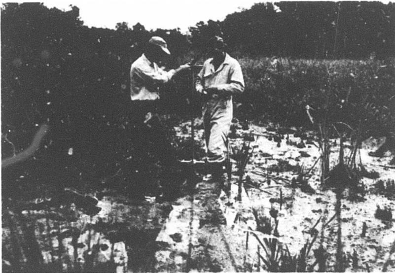
Fig. 13. Moisture-density sampling in muck
