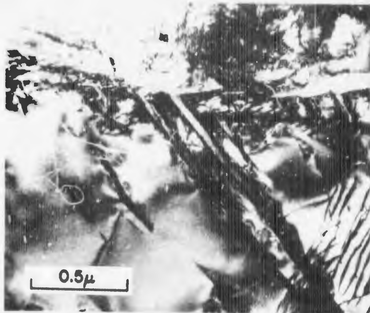
Fig. 10. The internal plates in the \alpha lath consist of a \beta strip bounded by interface phase, as illustrated here in Ti-6Al-6V-2Sn.
