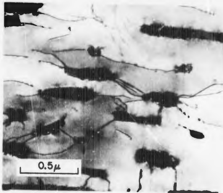
Fig. 18. Beta phase precipitates in large \alpha phase lath in Ti-6Al-4V, Condition E.
