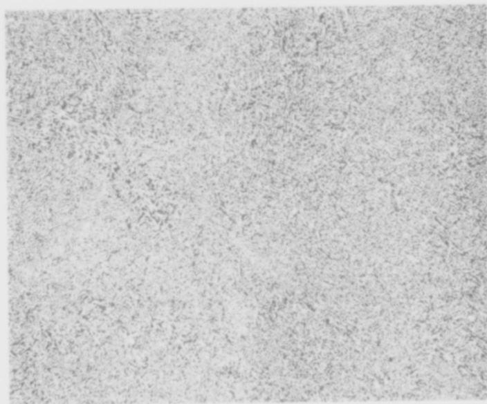
Item #9 Microstructure. Ti-6Al-2Sn-4Zr-6Mo 100 X 6 inch round coarse grained.
