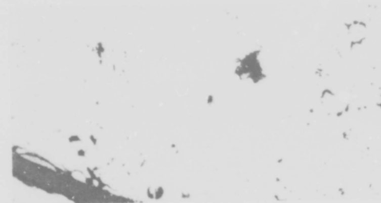
FIGURE 17. AS-POLISHED MICROSTRUCTURE OF ROD F-8 AT 4-3/16 - 4-13/16 IN. FROM BOTTOM OF FUEL COLUMN. Burnup 9,400 MWD/MTU.
