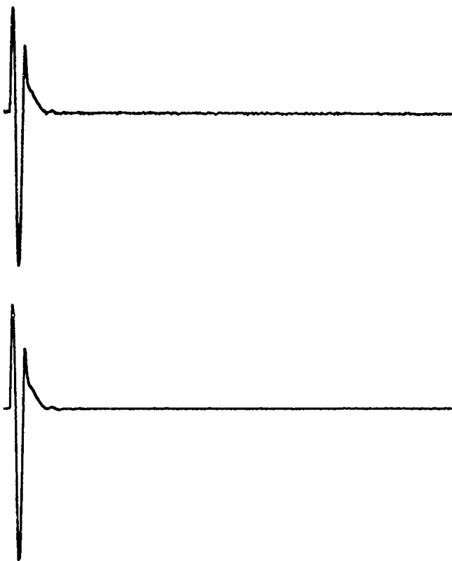
Fig. 10. J13 current waveforms, one cycle, 65-Hz signal. Top: raw J13 current waveform; duration, 0.5 s. Bottom: averaged J13 current waveform (100 waveforms used in average); duration, 0.5 s.
