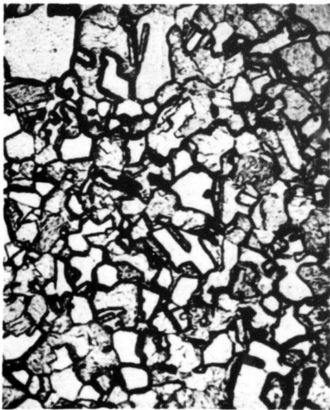
C. Surface View of Sample Ni-9 Showing Equiaxed Zone 2 Morphology. Deposition Temperature 426°C. (300X)
