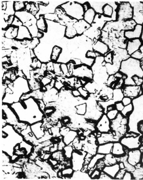
A. Surface View of Sample Ni-8 Showing Equiaxed Zone 3 Morphology. Deposition Temperature 554°C. (300X)
