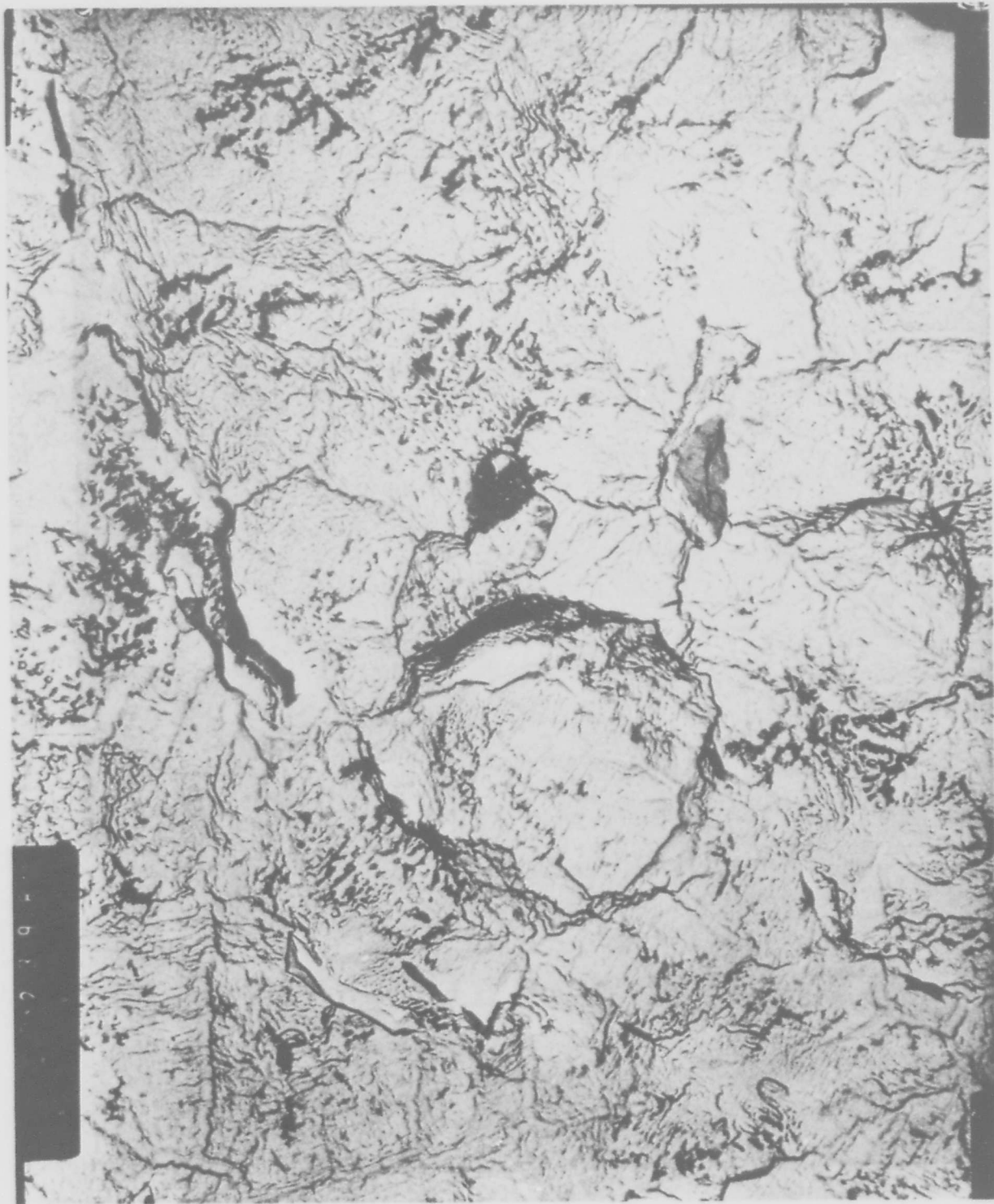
Fig. 62. Transmission electron micrograph of phosphate-fluoride film from Ti-6Al-4V.
