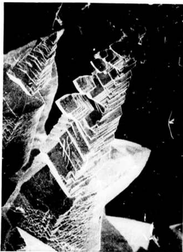
Figure 5a. Dendrites along [111] direction, composed of stacked cubes, evidence of corner growth, 180X.
