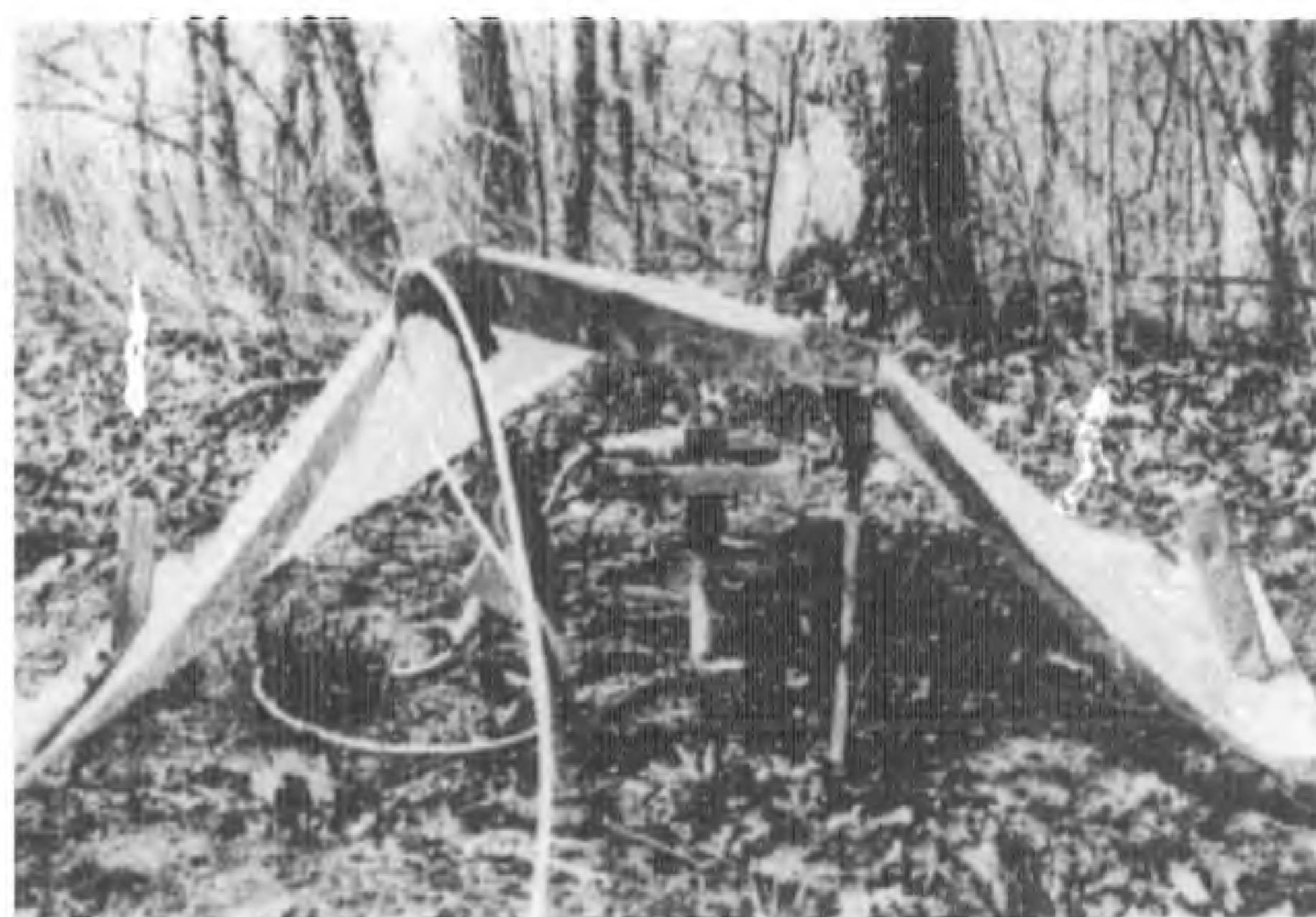
(b) Gage assembly under protective tent
