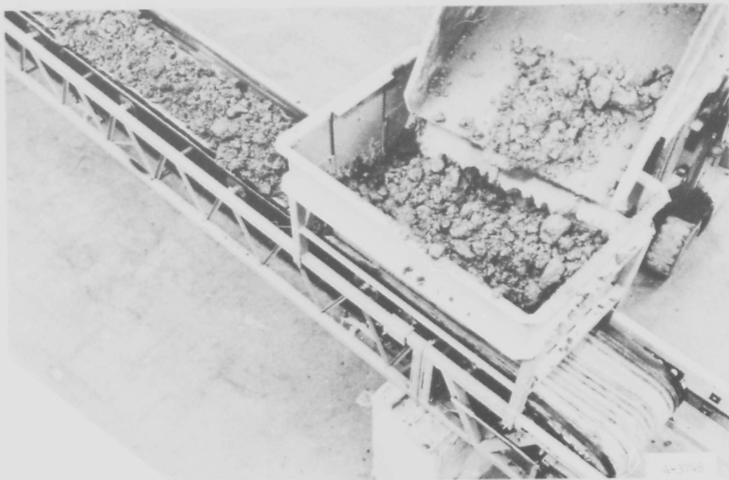
Figure 1. Type A belt used for transporting six-in. maximum-size aggregate concrete to test block
