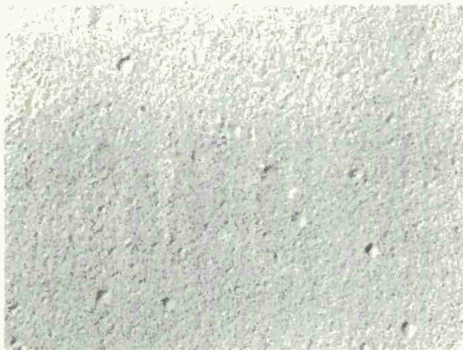
Figure 22. Electron micrograph of as-received bulk S-glass boiled 7 days in distilled water. No etchant. 39,900X
