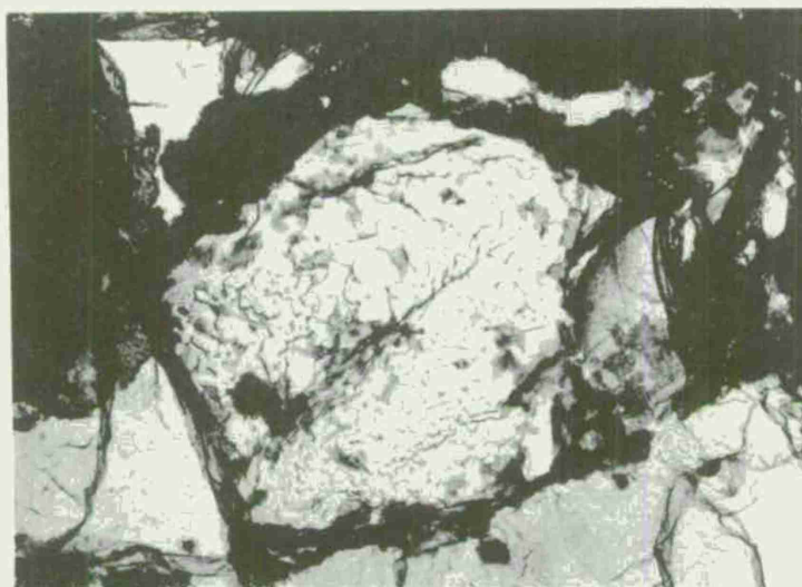
Figure 13. Electron micrograph of S-glass fiber cold mounted in epoxy, polished and etched 1 minute in 5% HF. 10,260X
