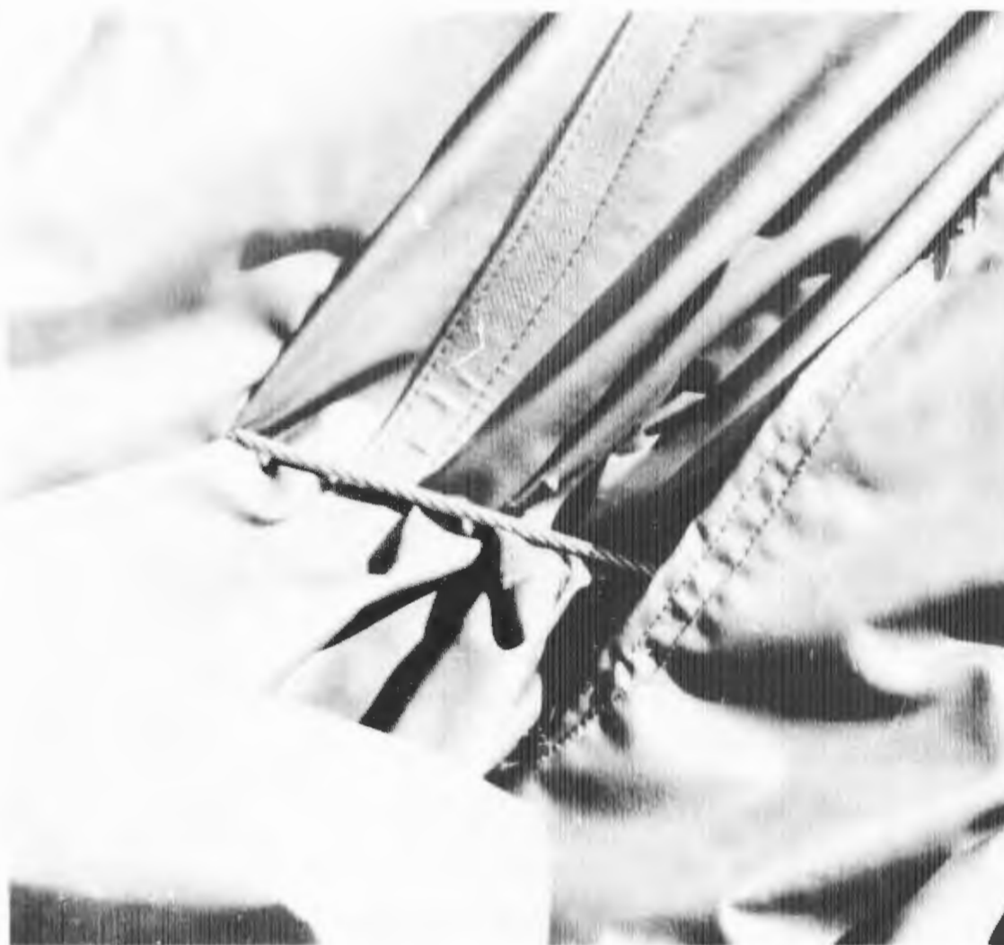
Figure 45 Cable Rubbing on Fabric as Door is Opened
