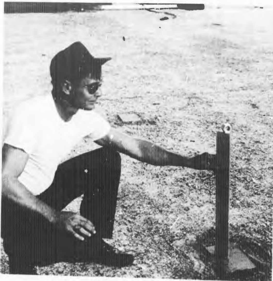
Figure 81 Measuring Height of Weights Before Load Test
