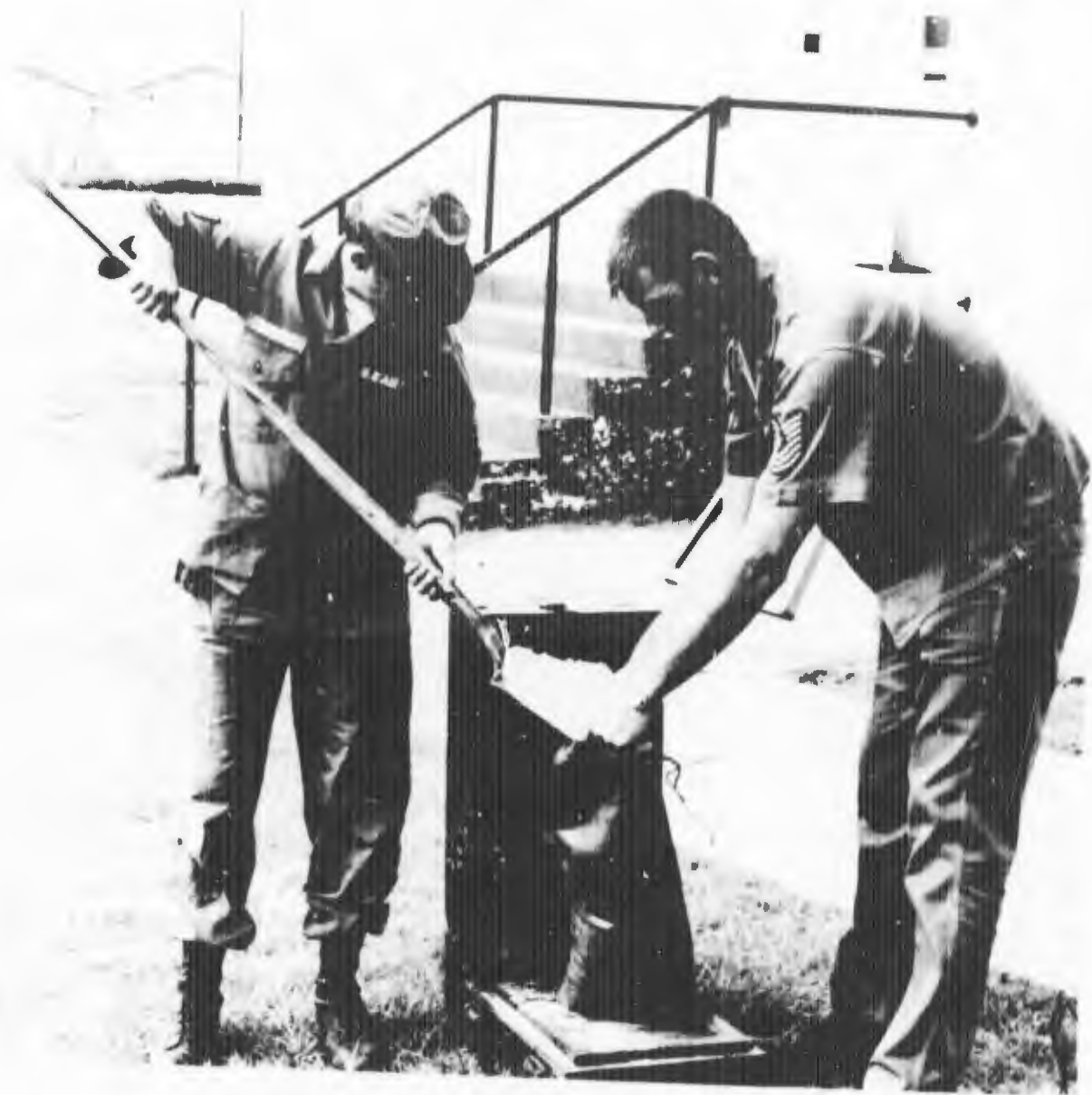
Figure 79 Weighing Sandbags for Load Test
