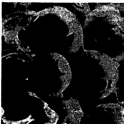
Fig. 14 -- Microphoto of zirconia stabilized spheroid-powder material [13]
