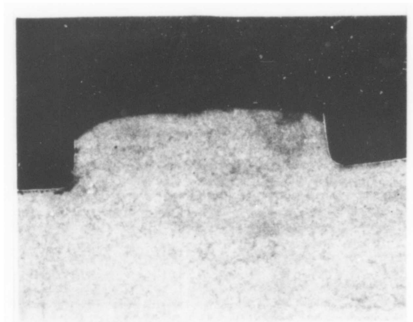
Fig. 37 Tube S.N.53; Section 3; 3 o'clock. Position of maximum wear (15 X).
