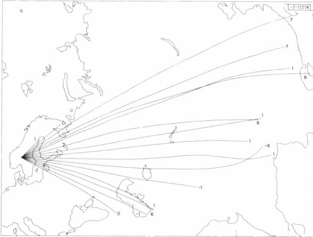
Fig. II-2. Ray paths traced from NORSAR (60.8°N, 10.8°E) at 5° increments in azimuth from 45° to 120°. Numbers at end of each ray give final azimuthal deviation. Longest ray is to 78° distance from NORSAR.
