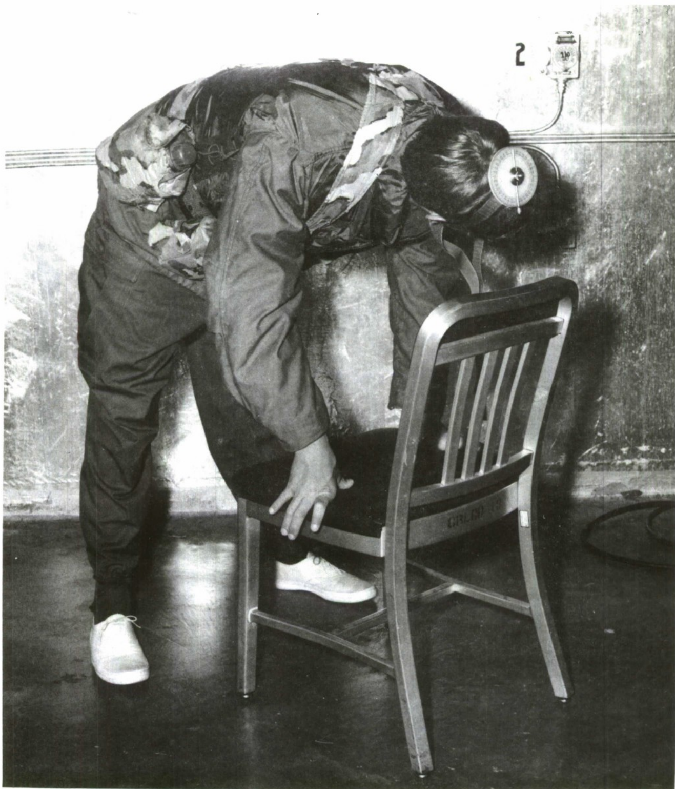
Figure B3. Head Rotation. Goniometer set to zero.
