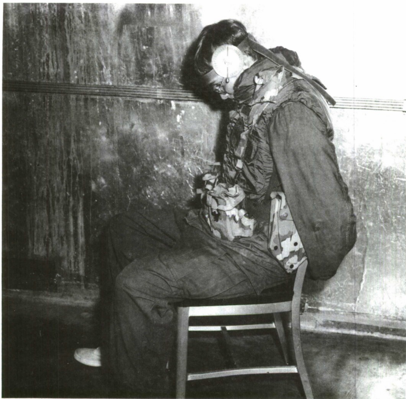
Figure B1. Head Movement, Ventral to Dorsal. Goniometer set to zero.
