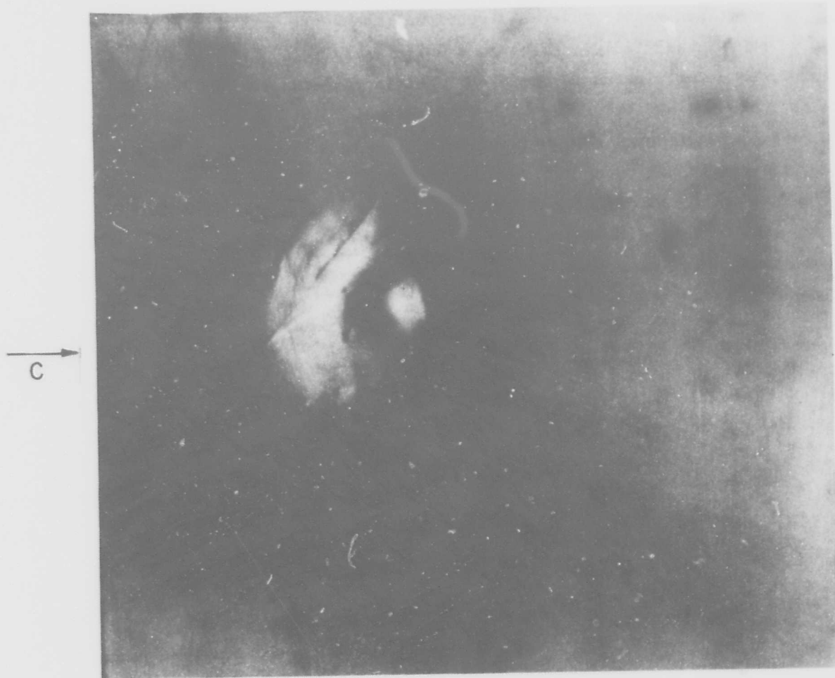
Figure 6. Photograph of Fe-doped \text{LiNbO}_3 after extended exposure to 4880 \text{ \AA} argon laser beam. The dark coloration is on the +c side of the illuminated region.
