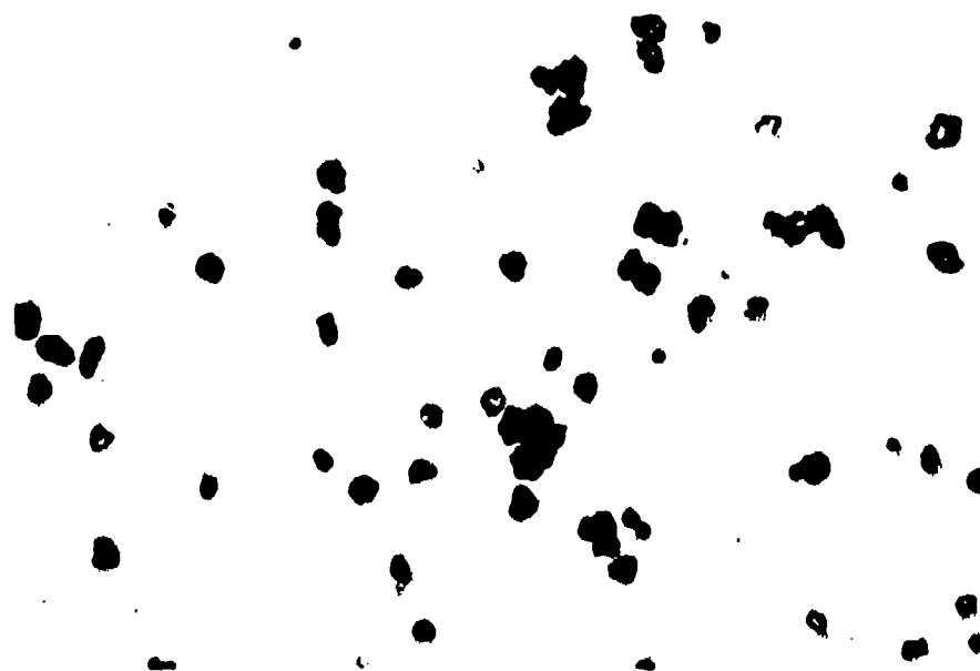
Figure 15. Particles collected at 3.60 \ell/\text{min.} , maximum equivalent diameter = 2.0\ \mu\text{m} (1000X)
