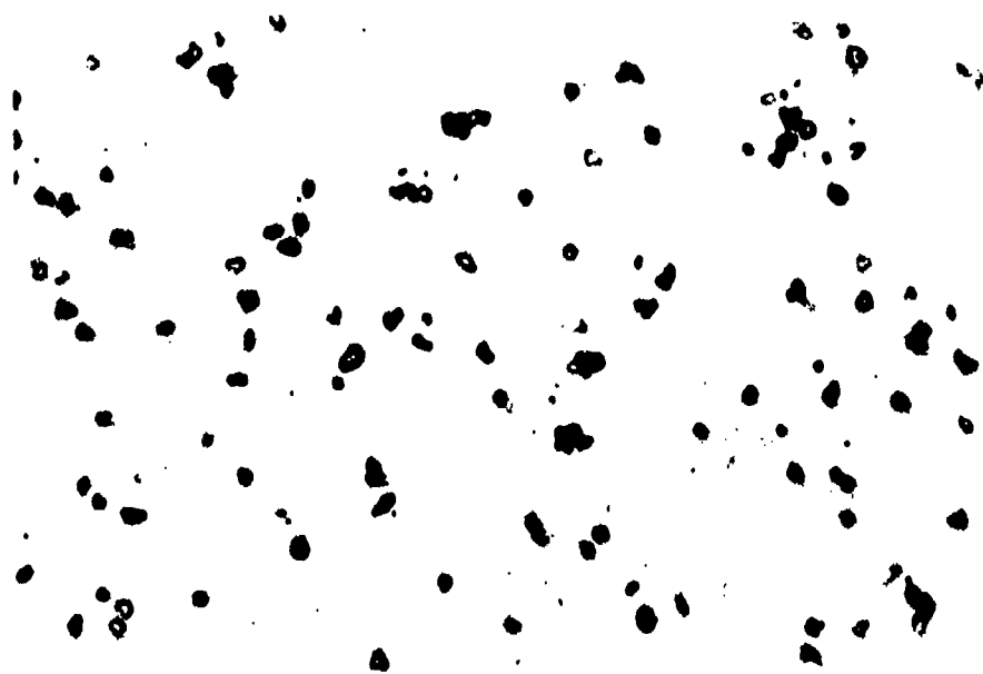
Figure 14. Particles collected at 7.19 \ell/\text{min.} , maximum equivalent diameter = 1.2\ \mu\text{m} (1000X)
