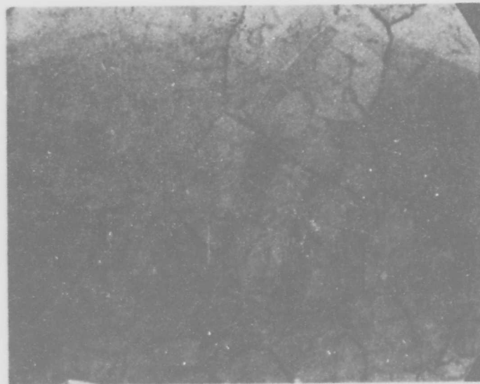
Figure 22. Vendor A Material Heat Treated for Two Hours at 1050°C (Heat Tinted), Mag. 375X
