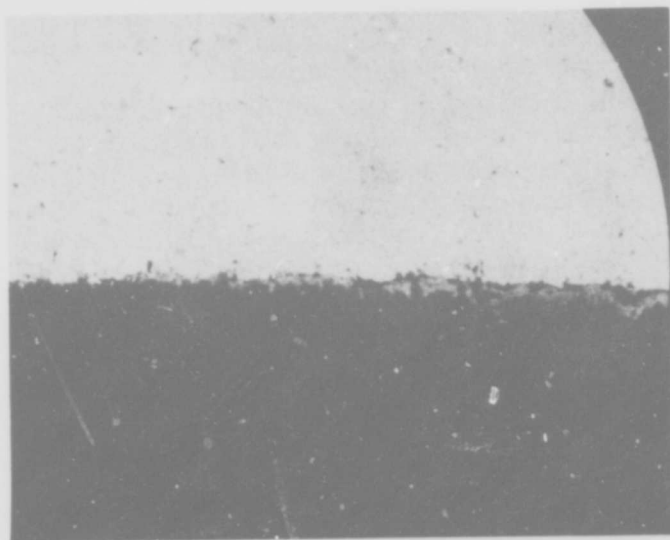
(b) Good Seal -- Oxidized at 750^{\circ}\text{C} , Dried Air, 40 Minutes, -56^{\circ}\text{C} D.P., Sealed at 950^{\circ}\text{C} , 15 Minutes, Mag. 350X
