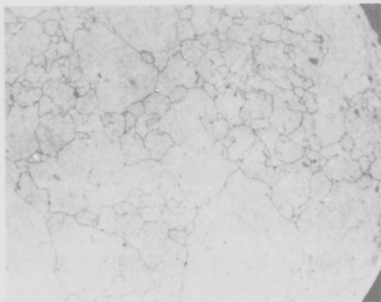
Vendor B Material, Below Surface of Sheet, Mag. 375X
