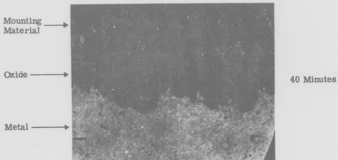
Figure 8. Vendor A Material Oxidized at Three Different Temperatures (20 CFH Dried Air, -56°C Dew Point, Mag. 350X) (Sheet 1 of 3 Sheets)
