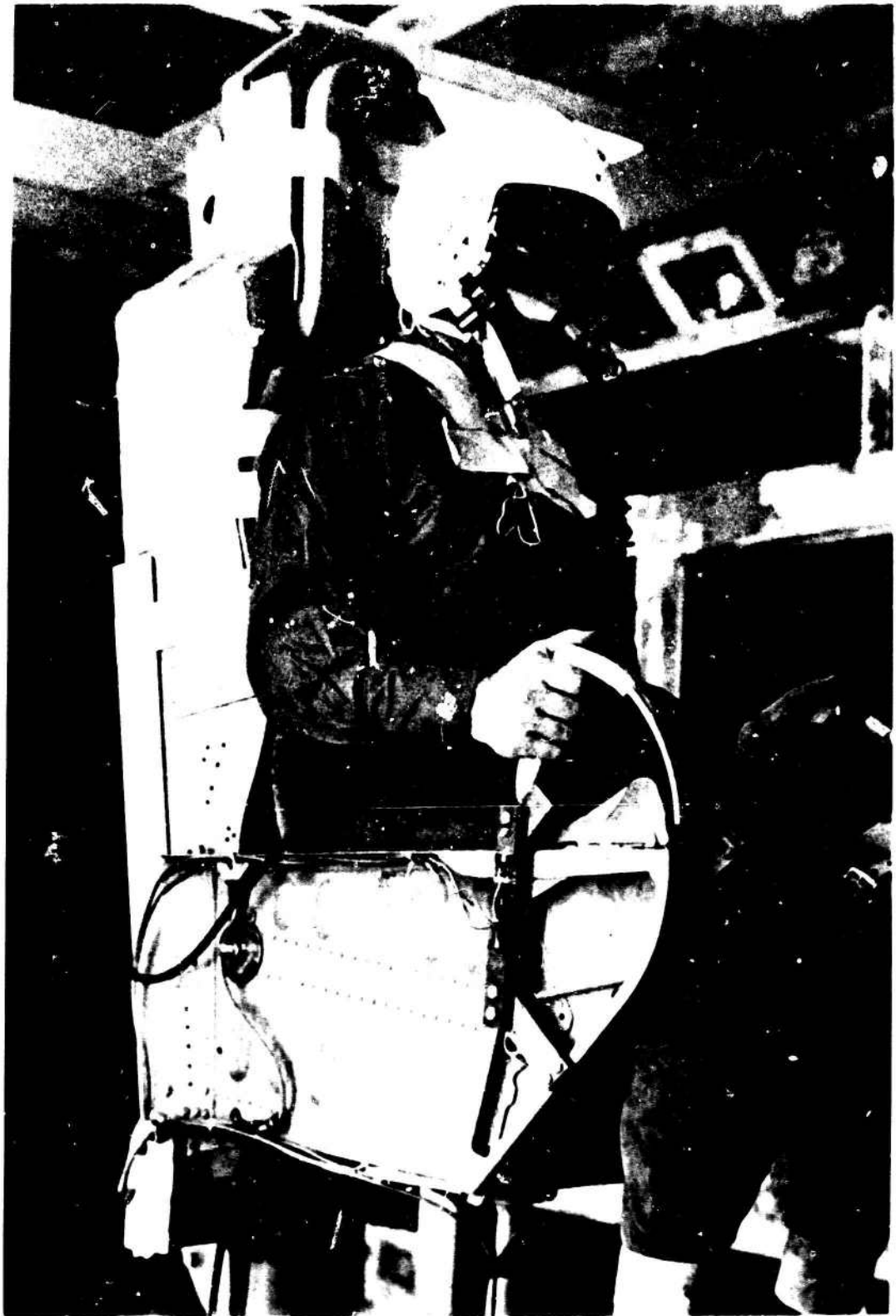
Figure 10. The ACES-II Side Arm Control Handles were Mounted on Strain-Gauged Cantilever Beams Which Permit "in-out" and "Forward-Back" Forces to be Measured.
