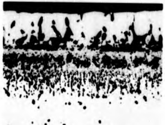
Figure 45.16. Udimet 500 with only 7% Cr after oxidation for 3 days at 1000°C in air. Magnification 460X. (Seybolt).
