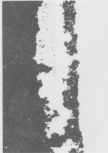
Figure 4.2. Deterioration of aluminized coating on a G.64 turbine rotor blade after 3000 hr running. (Llewellyn).
