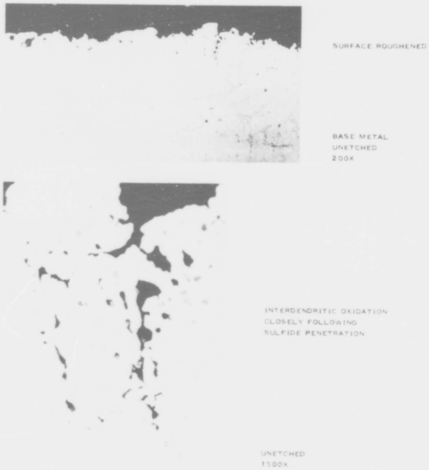
Figure 51.6. Hot corrosion of WI-52 in Phillips Rig. (Schirmer and Quigg).
