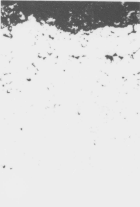
Figure 52.5. The extent of the internal oxidation of X-40 after 100h at 1800°F (982°C). X500, taper section x3.5. (Wlodek).
