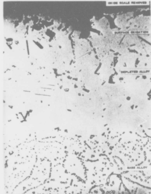
METALLOGRAPHIC CROSS-SECTION OF INCONEL 713C SPECIMEN AFTER 55 HOURS AT 2000°F TEST CONDITION. ELECTRO-CLEANED. MARBLE'S REAGENT ETCHED. 1000X MAGNIFICATION.
