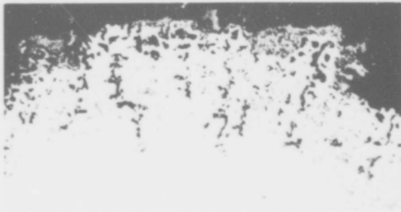
Figure 51.13. Subsurface oxides (dark gray) and chromium-rich sulphides (medium gray) in WI-52 tested in G.E. small burner rig at 1900°F (1038°C). (Bergman et al).
