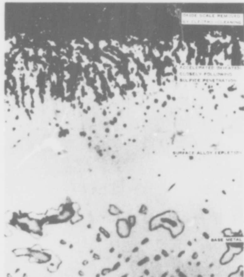
Figure 10.28. Hot Corrosion of Inconel 713C Specimen (Quigg and Schirmer).
