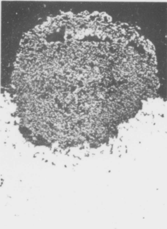
Figure 52.7. Localized catastrophic oxidation in X-40 after 100 hours at 2000°F. (Wlodek). Unetched X100.
