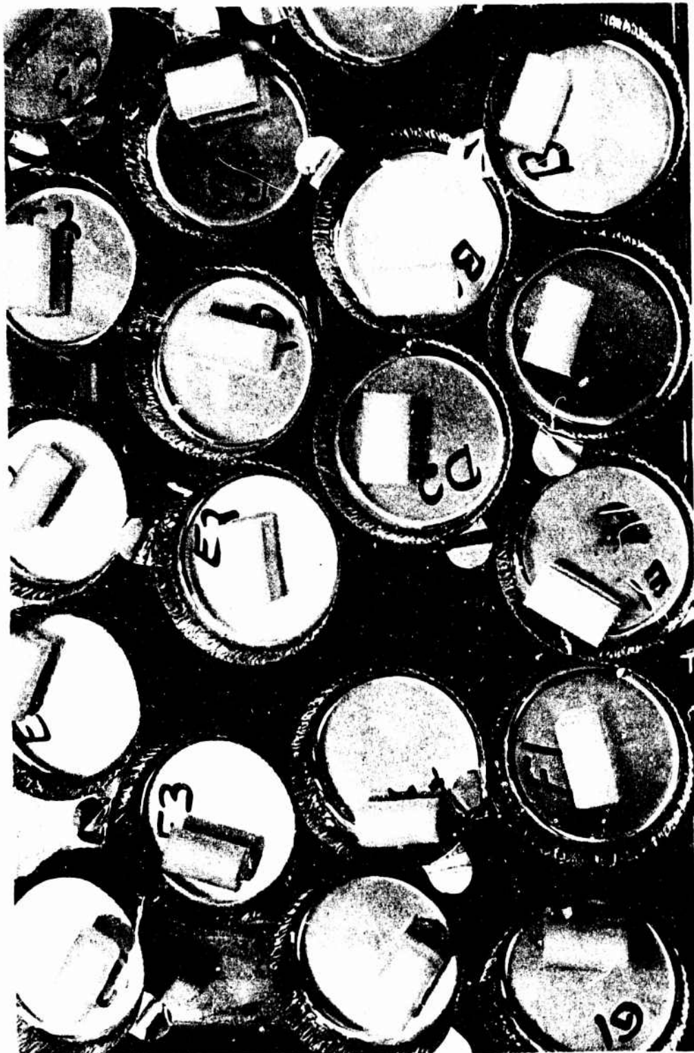
FIGURE 32 - LOOSE-FILL SPECIMENS PRIOR TO 31 DAY HUMIDITY TEST
