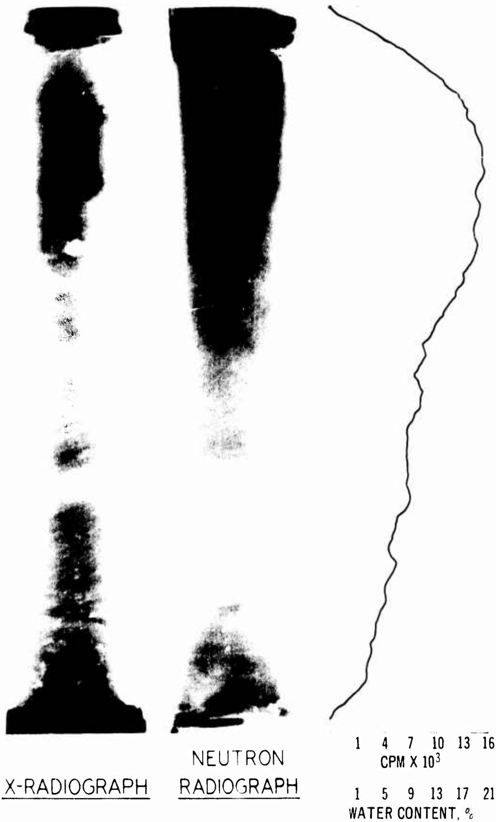
Figure 17. Radiographs of steel-encased 3-in.-diam soil sample. Graphic illustration at right was determined through neutron scan of core
