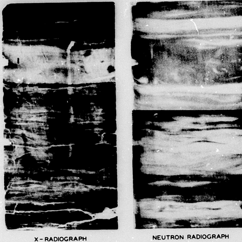
Figure 12. Comparison of X-ray and neutron absorption in 3/8-in.-thick soil slab
