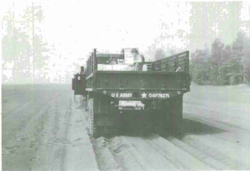
Figure 5. Drum and wire line system for measuring test vehicle speed.
