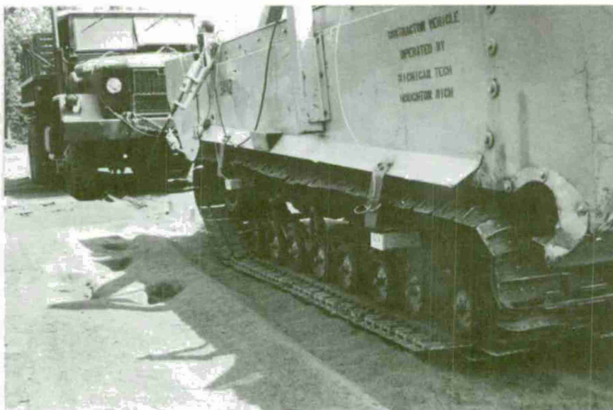
Figure 4. Drive sprocket tachometer-generator and chassis to suspension sinkage measuring pots.
