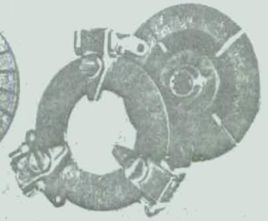
Model TS Single plate, dry; 5 1/2, 6, 6 1/2 in.; 50 to 75 ft. lb. max. capacity. Used in midget cars and trucks, small garden tractors, and auxiliary drives in industrial trucks.
