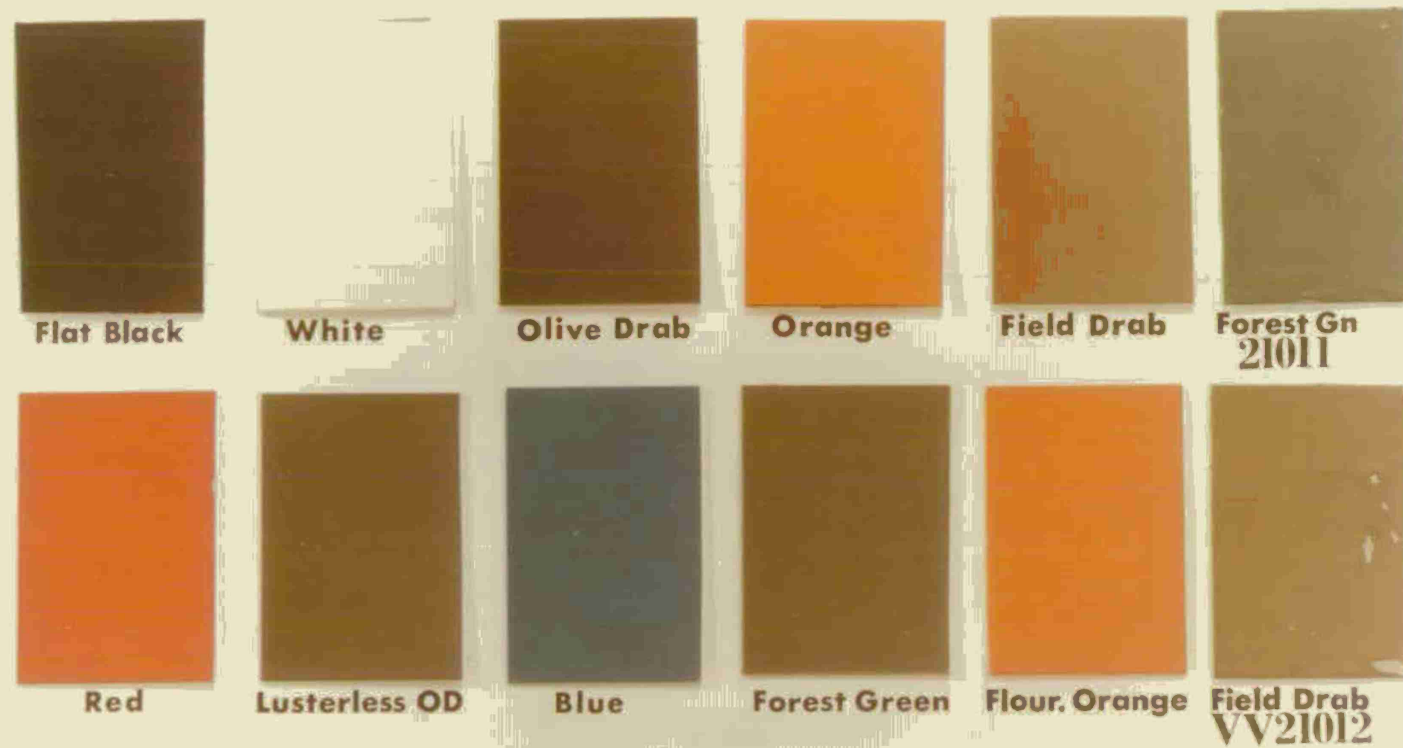
Figure 1. Paint samples used in the experiments. All of the colors are reproduced fairly well with the exception of red and fluorescent orange, both of which appear considerably brighter to the eye.
