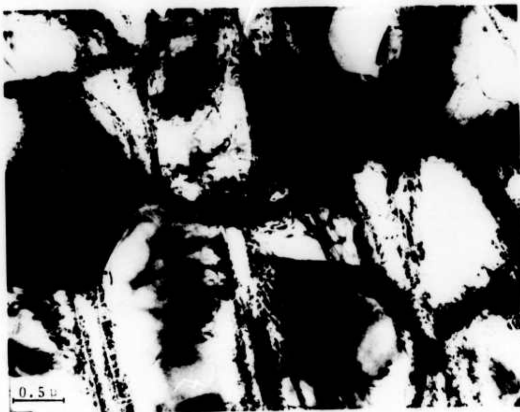
Figure 6. Transmission electron micrograph of a specimen \alpha - \beta annealed.
