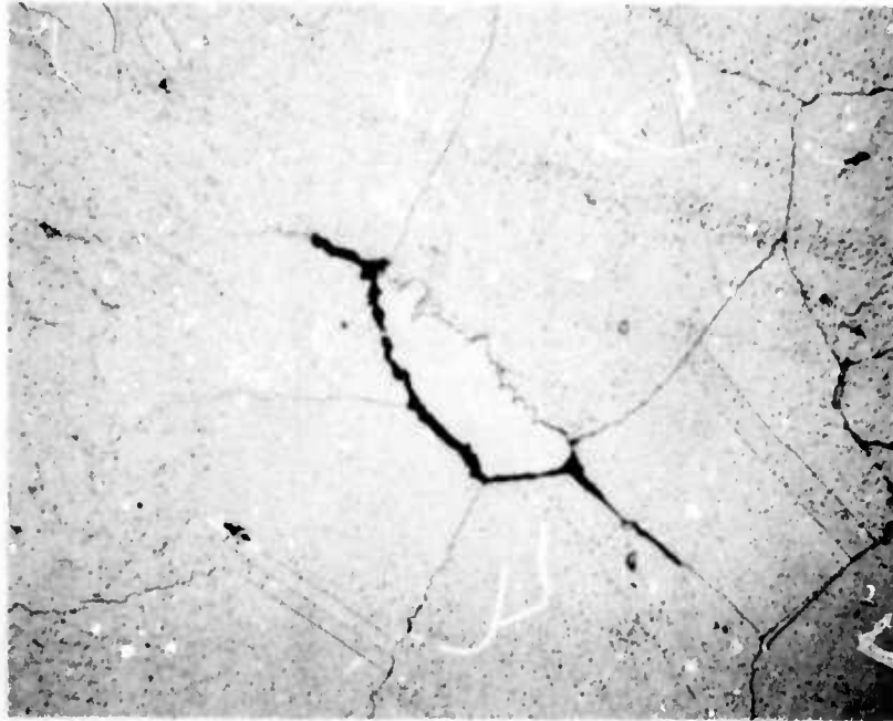
Figure 1 - Typical microfissure observed along grain boundaries in HAZ immediately adjacent to the weld fusion line in vacuum EB welded IN X750, (X200).
