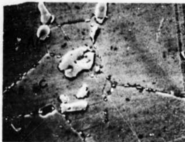
Fig. 14-I-718, as received. SEM micrographs (a) 150X (b) 300X c: 1500X. Energy dispersive X-ray analyses of points in (c) are shown in Figure 15
