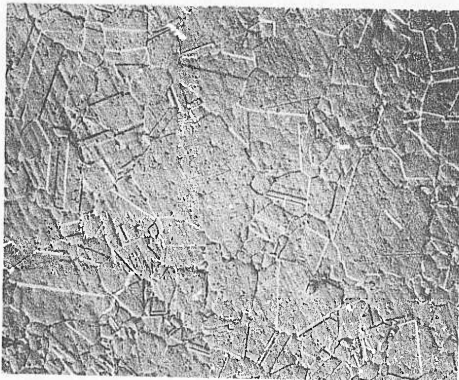
Figure II-4 Microstructure of 21-6-9 Annealed Stainless Steel
