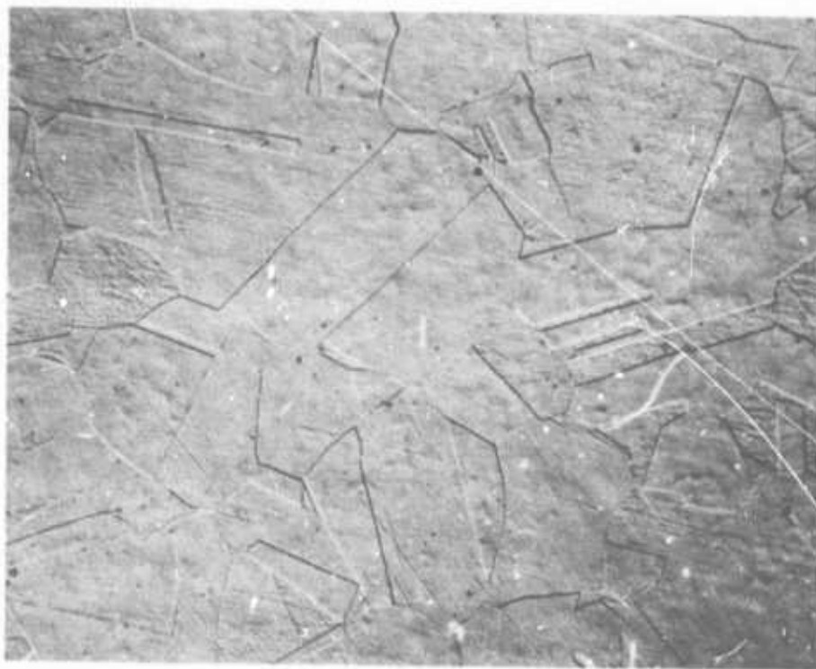
Figure II-2 Microstructure of 304L Annealed Stainless Steel
