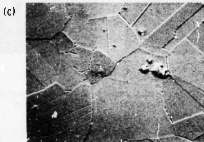
Fig. 43—SEM micrographs I-706 (a) VIM-VAR, S. A 2100°F (1422°K) 2 hr, 650X (b) VIM-VAR, STDA (71 XX) 200X (c) VIM-EFR, STDA (70XX) 1250X
