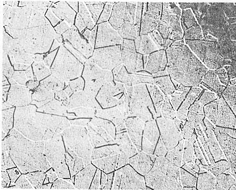
Figure II-5 Microstructure of A-286 Solution Treated and Aged Stainless Steel
