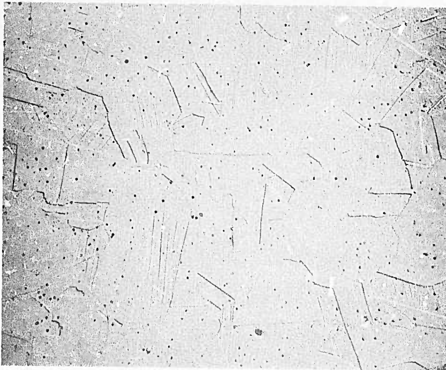
Figure II-3 Microstructure of 310 Annealed Stainless Steel
