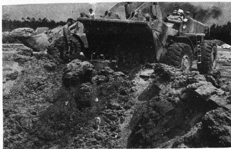
Figure 47A. Test 1-2, Operation of AC 745 Loader with Four in One Bucket in Closed Position
