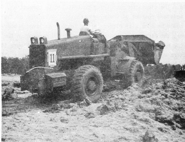
Figure 12. Test 1-1, AC 645 Loader Forced to Lift and Drop Debris into Crater
