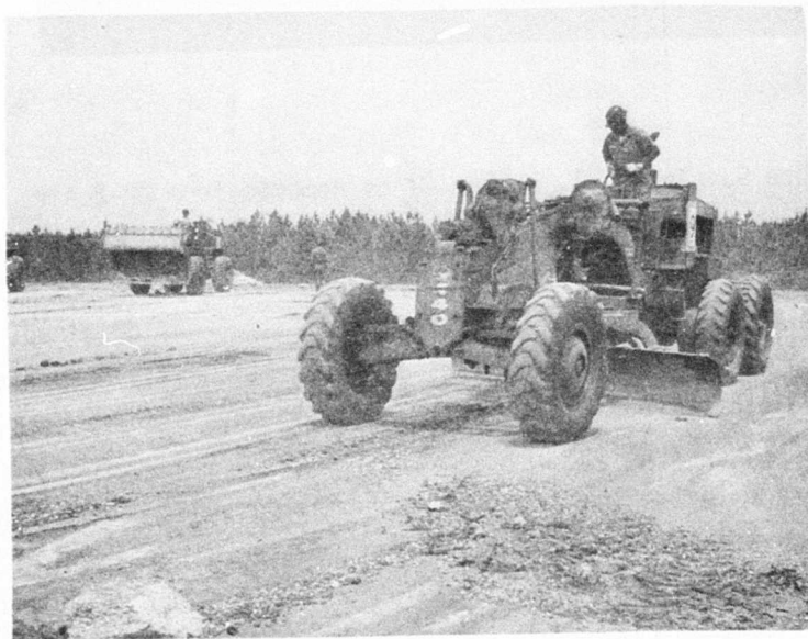
Figure 10. Test 1-1, Motorized Grader Cleaning Small Debris from AM-2 Air Field
