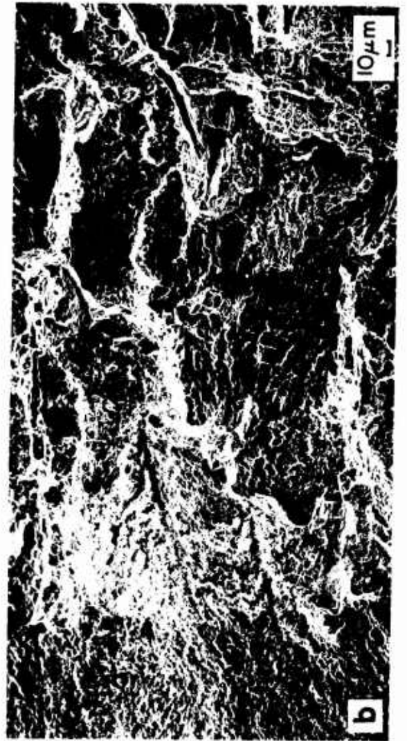
Figure 166. Alloy 334, sample 4SLC2. SEM of fracture surface (a) X25, (b) X250-precrack/fast fracture transition, (c) X250, (d) X500 - fast fracture.
