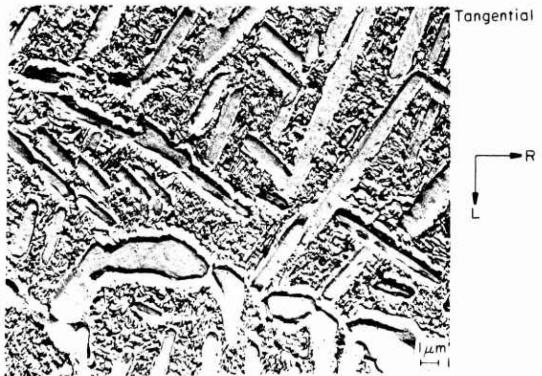
Figure 177. Alloy 227(7Mo-4Cr-2.5Al). Six inch billet full piece, center samples 7SLC1 and 7LRC2 (Table LXVII). Solution annealed 1450F-2 hr WQ plus 1350F-8 hr WQ, aged 925F-8 hr. Isometric X100, surface replica X5200. YS(ksi): 151 (L) RA(%): 36 (L) K Q (ksi/in): 84 (LR) 152 (T) 18 (T) 50 (SL)
