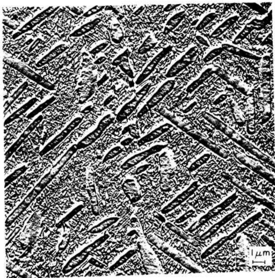
Figure 187. Alloy 227, sample 7SLE2. Fracture surface X8, surface replica X5200.
