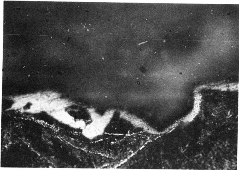
Fracture path from above. Crack propagated left to right. X500
