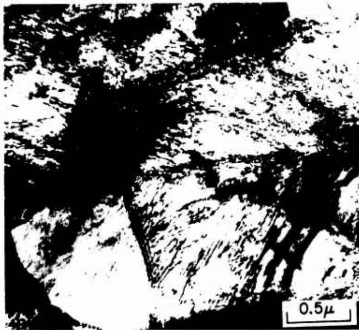
Fig. 70 Transmission micrograph of Alloy 266 (11Mo-4Al) as solution treated revealing sub-grain structure in \beta matrix.
