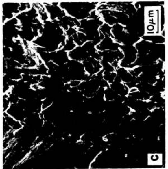
Figure 127. Alloy 253, sample 3ESR2. SEM of fracture surface (a) X25, (b) X300, (c) X1000- precrack/fast fracture transition, (d) X300, (e) X1000-fast fracture.
