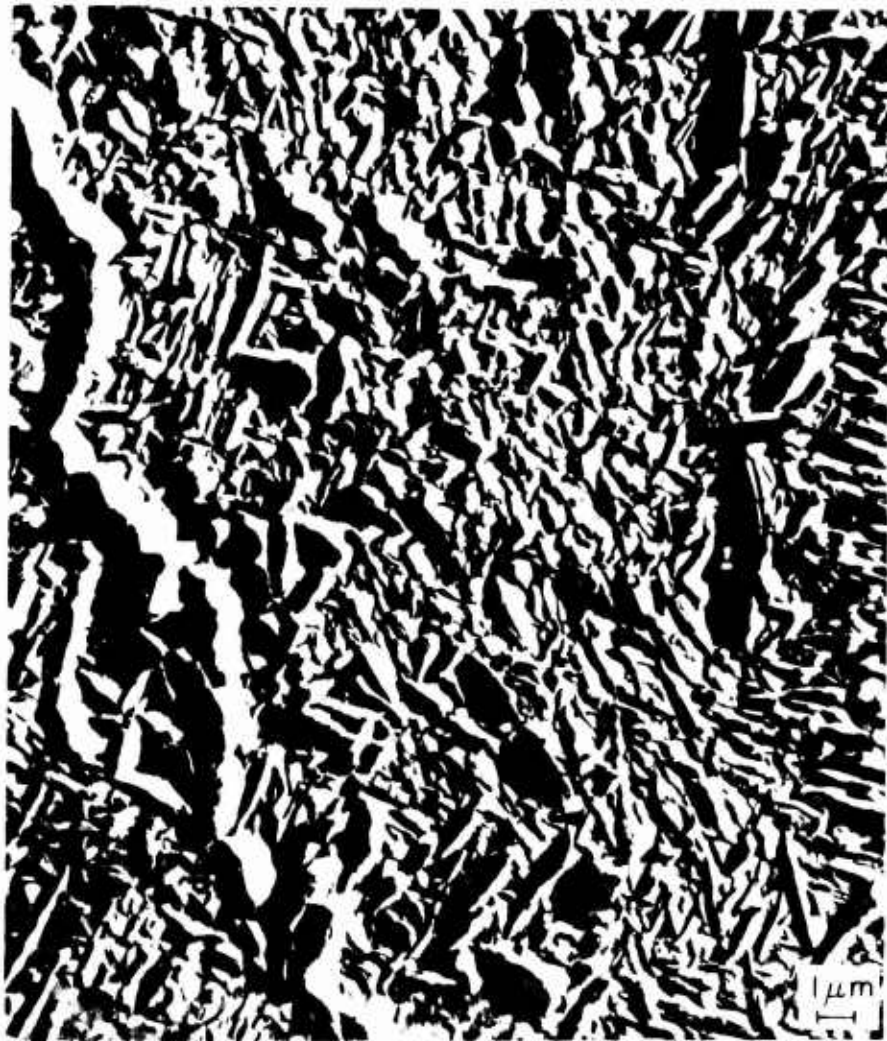
Figure 169. Alloy 334, sample 4LRC2. Surface replica X5200.
