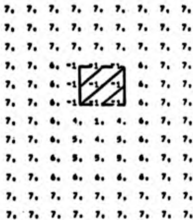
Figure 8. A numerically simulated sea height depiction (ft) at hour 39 for a surface wind speed of 7\frac{1}{2} m sec -1 ( 2\frac{1}{2} m sec -1 in lee of island). Sea heights shown are average values for the highest 10% of The swell ( H/10 ). Average swell height ( H ) is H/10 \div 2.03 .
