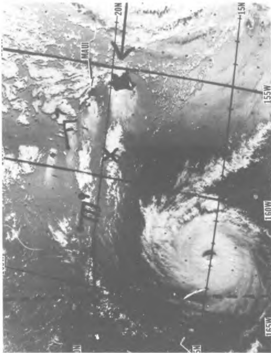
Figure 17. A DMSP VHR visual depiction on 17 August 1972 at 1917 GMT. The dashed line is the sub-satellite track. The circle on the track represents the sub-satellite point. The line through the circle represents a scan line. The specular point location is denoted by an X. The arrow is on the great circle arc connecting the subsolar point, and the sub-satellite point. Subsolar point location is 13.2 N/108.3 W. Wind reports are in knots (1 barb = 10 kt). Hurricane Celeste (intensity 85 kt) appears SW of the island chain.
