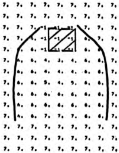
Figure 14. A numerical simulation of swell height at hour 15 under wind speed conditions of 7-1/2 m sec -1 . Sea heights shown are average values for the highest 10% of the swell (H 1/10). Average swell height (H) is H 1/10 = 2.03.
