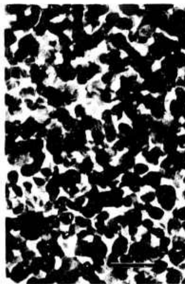
d. Heat Treated for 2 hr at 750°C. Layered structure completely absent. Mo spheres (dark phase) are \approx 860 \text{ \AA} in diameter. 51,000X
