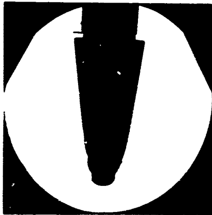
Run 822 1.5-inch, R_s Laminar-Blunt Re_{\infty} = 4.02 \times 10^6/\text{ft} , T_o = 960^\circ\text{F}
