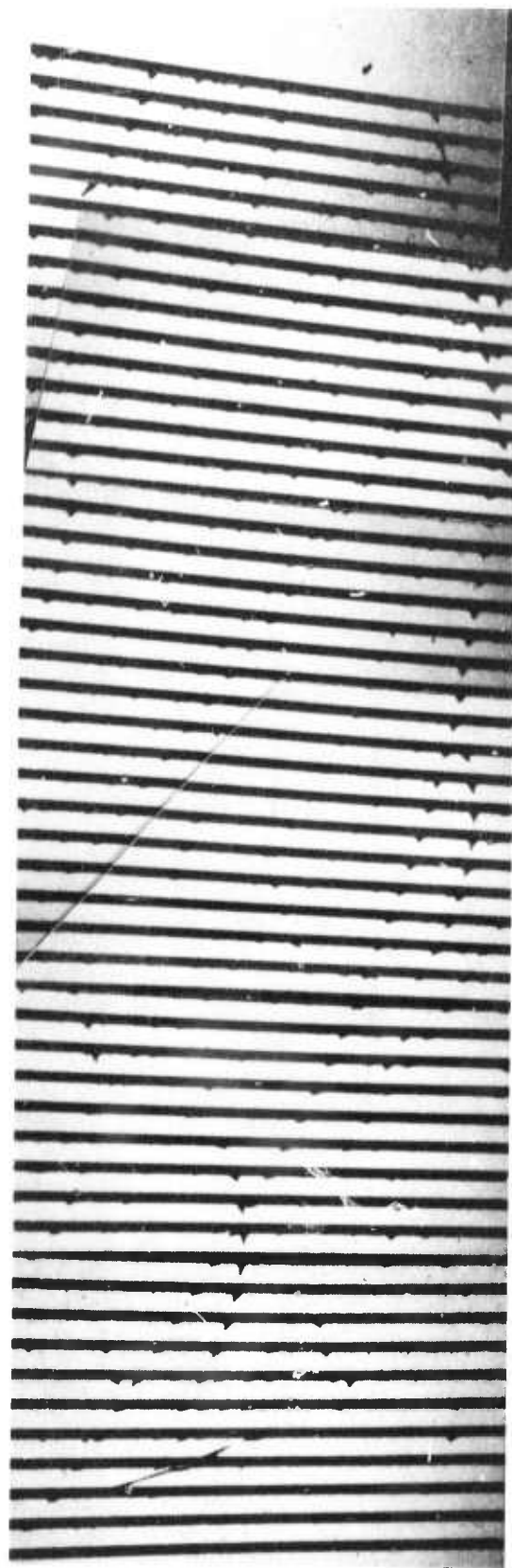
Figure 11 Polishing Damage in a Field of Etched \text{LinbO}_3 Waveguides. Lower photograph at \sim 100\text{X} . Upper left- and right-hand photographs at \sim 250\text{X} and \sim 500\text{X} , respectively.
