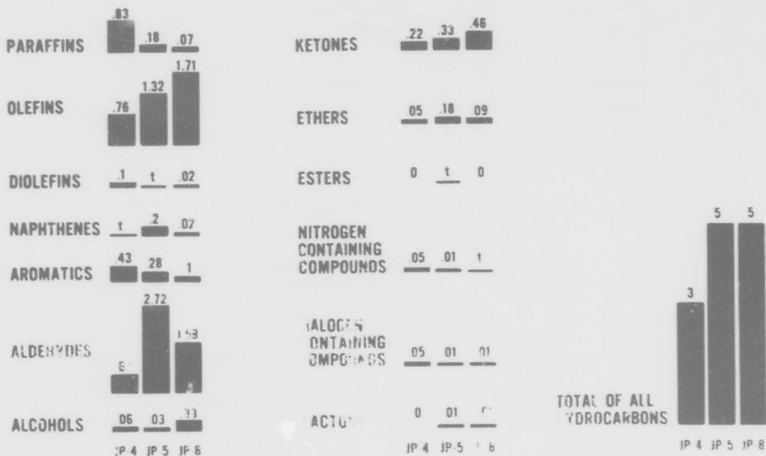
Figure 6. Exhaust Hydrocarbon Concentration (ppm) as Benzene with Various Fuels at 33 psig Inlet Pressure
