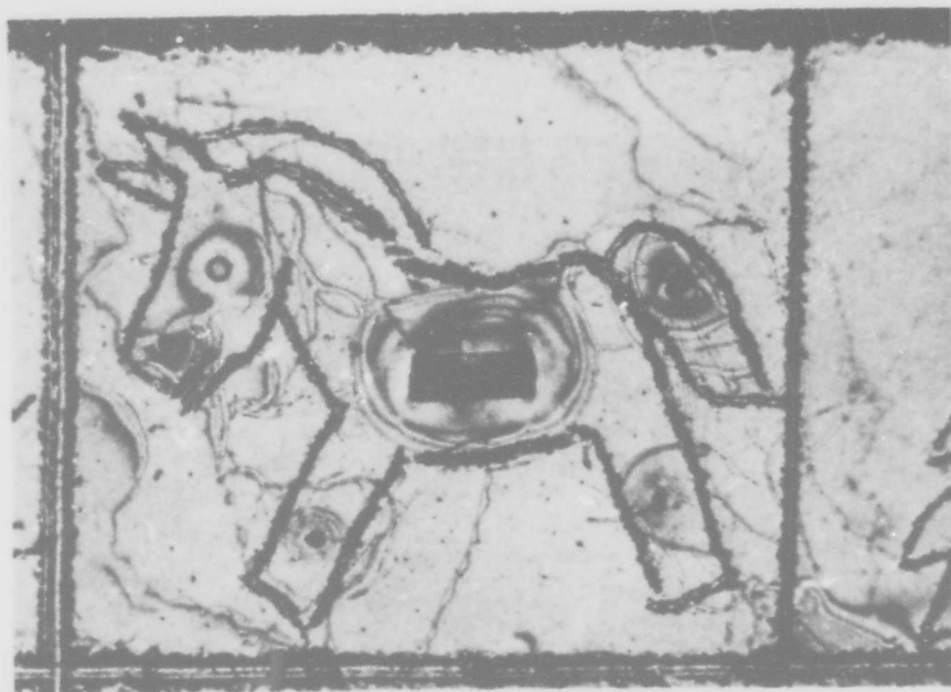
Figure 7. Two Pictures Drawn on Highly Polished Beryllium Plate as Keys to Location of Particles for Probe Analysis, Brightfield Top Light, 200X
