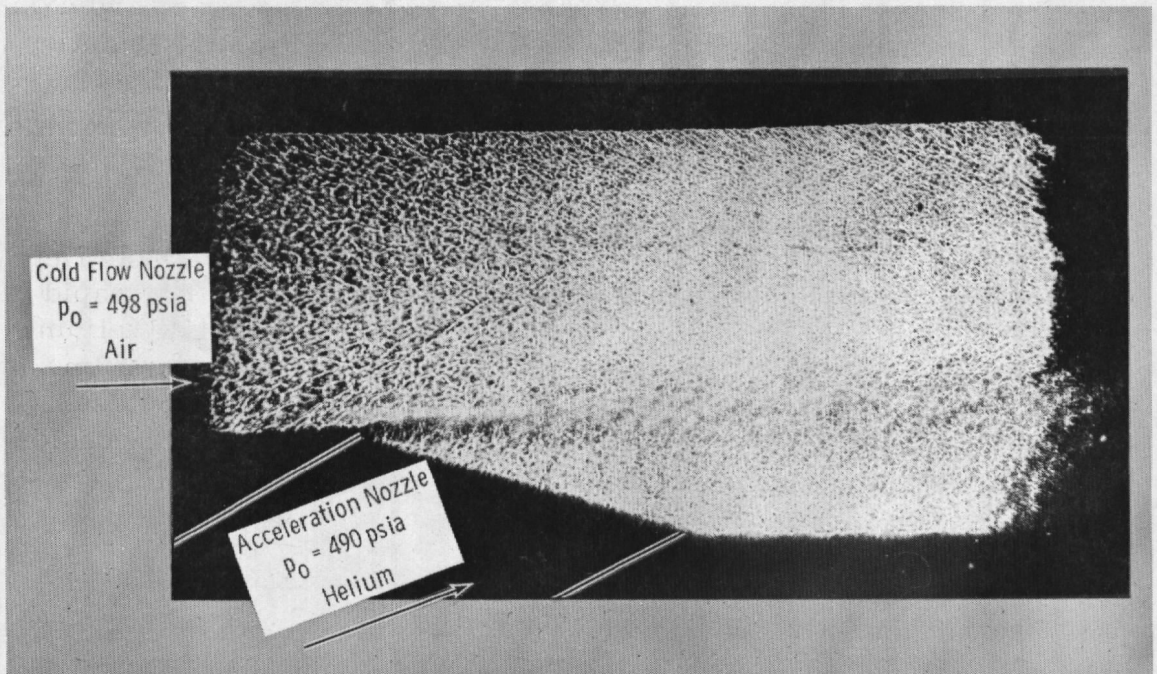
Figure 30. Shadowgram of flow in cold-flow nozzle, no skimmers.
