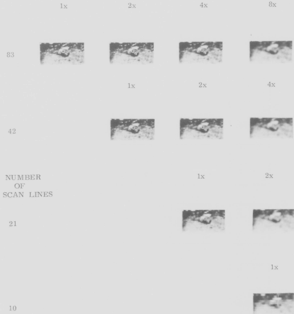
Figure 31. A jeep degraded under the ten combinations of number of scan lines and scan aperture size.
