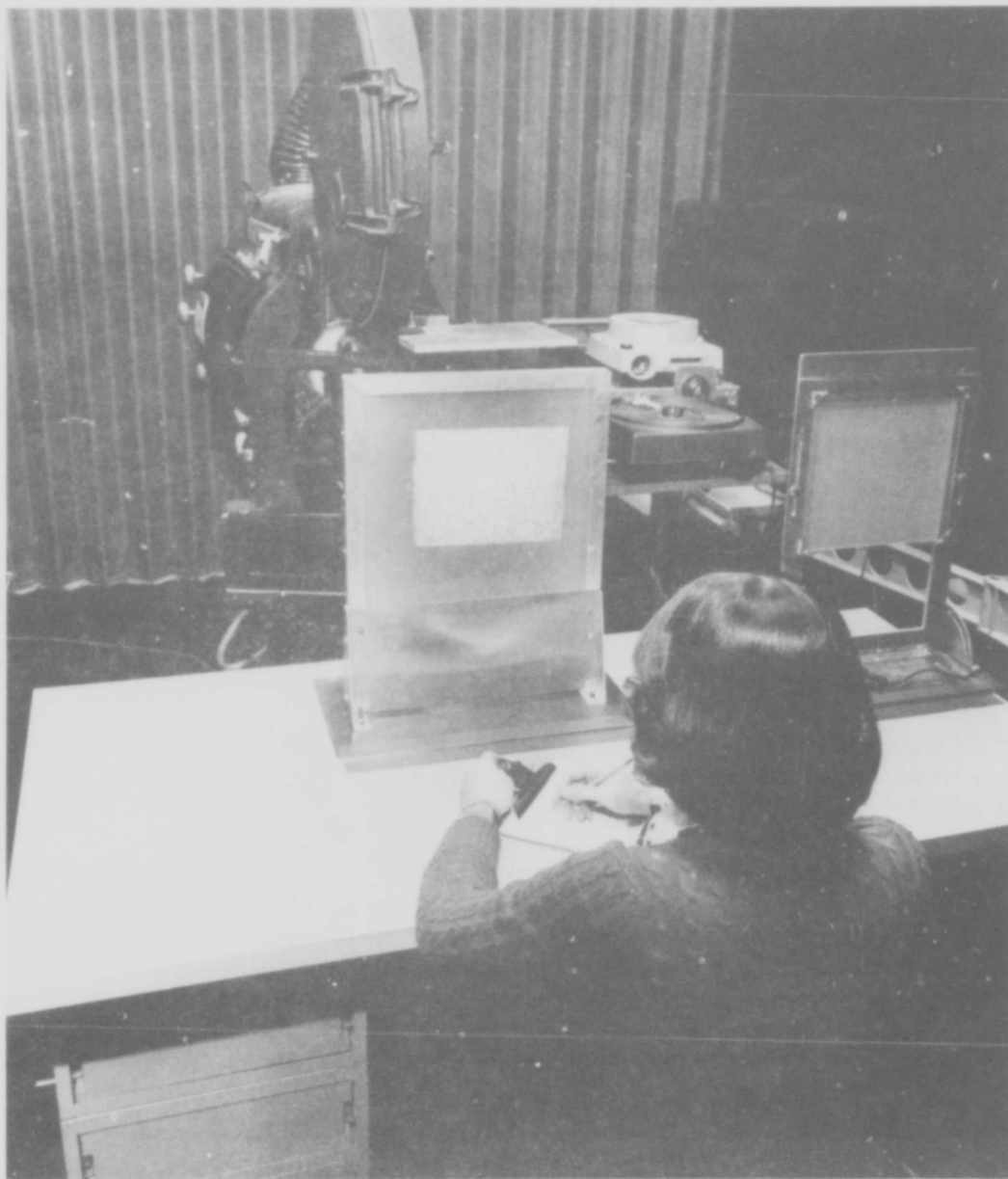
Figure 55. The experimental apparatus (from left to right): 35 mm movie projector; rear projection screen; background projector; training slide projector; training rear projection screen.
