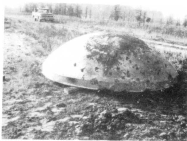
Figure 13. Cumulative damage on 6-in. dome from 81-mm mortars detonated at 5, 10, and 15 ft.
