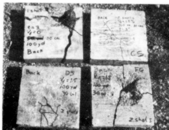
Figure 31. Scabbing from a 30-caliber machine gun of 3-in. plates with differing fibers.
