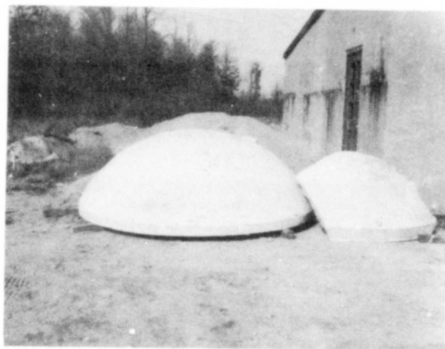
Figure 18. 4\frac{1}{2} -in. nominal thickness dome and portion of 6-in.-thick dome used for 50-caliber and 20-mm tests.
