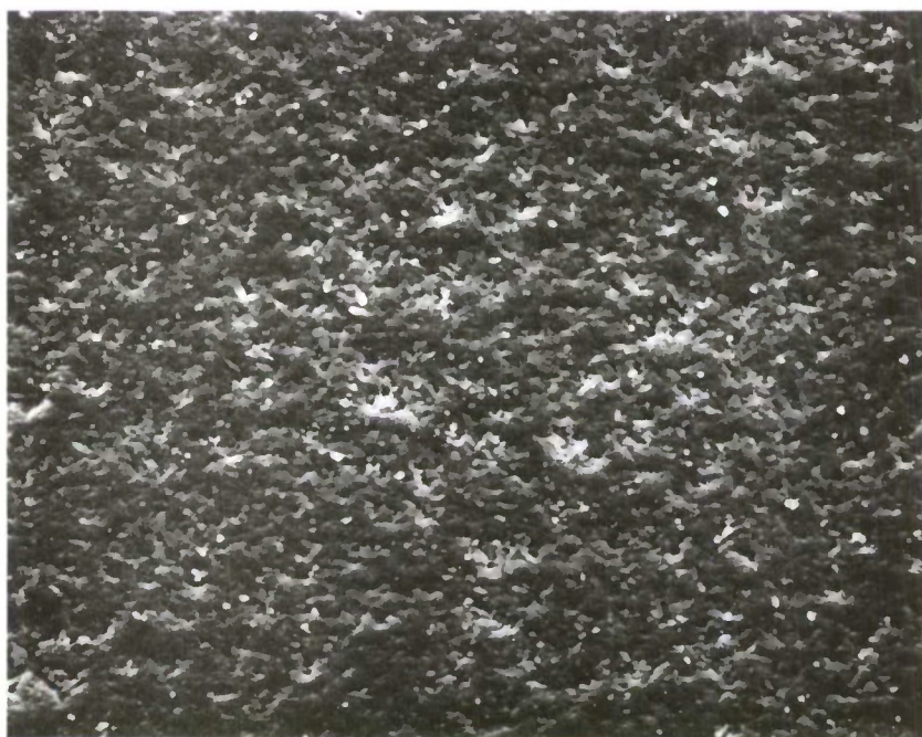
FIGURE 21 - Appearance of diamond grit lapped surface after RCF test, 1000X.
