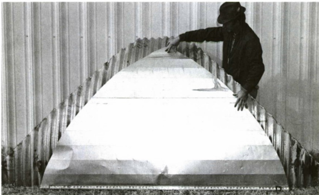
b. Quarter-section template of MICS showing ample material available for fabricating an additional quarter-section
