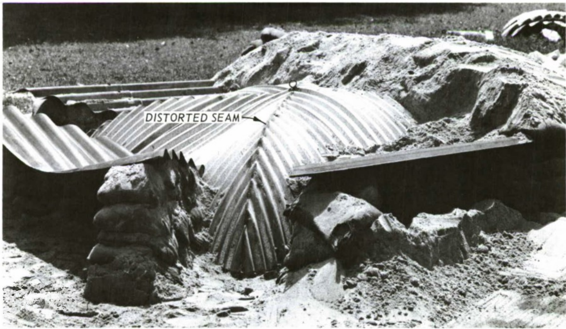
d. Typical distorted seam
