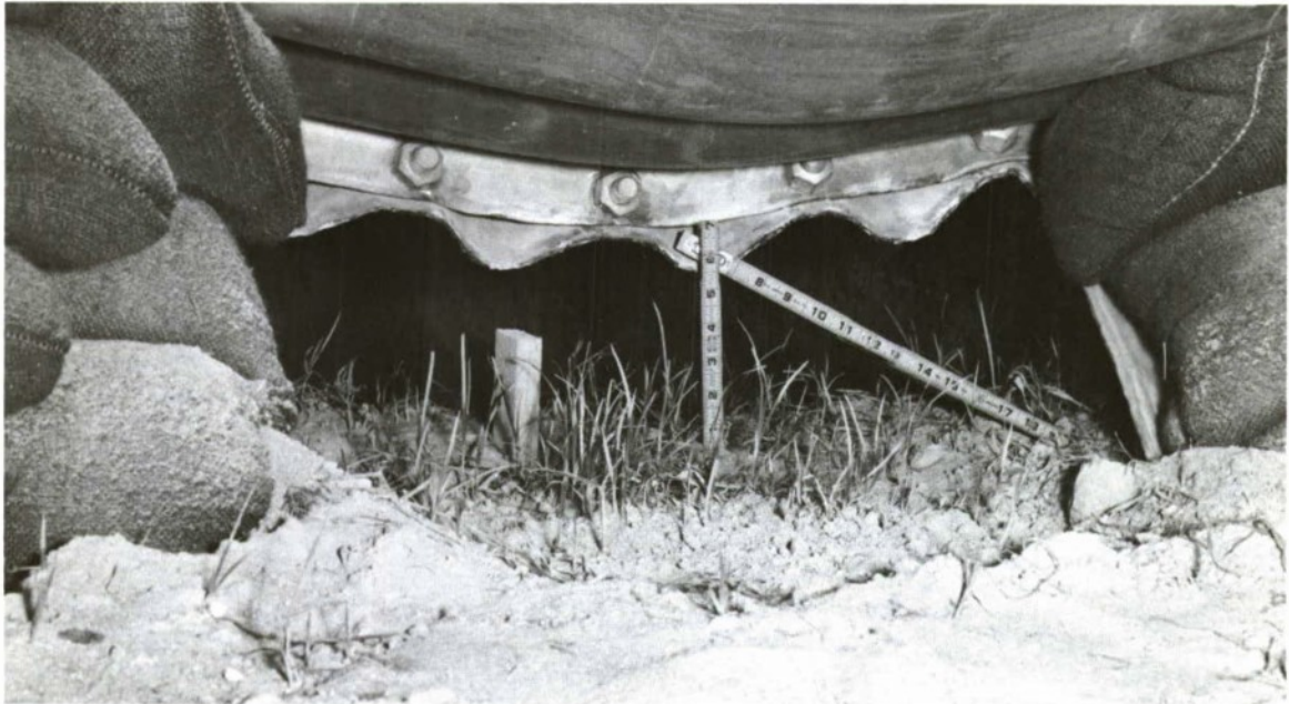
c. Aperture on loaded side of MICS
