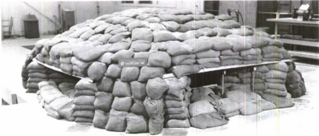
d. Four layers of sandbags
