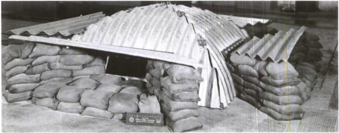
a. Test structure with six layers of sandbags supporting the aperture beams
