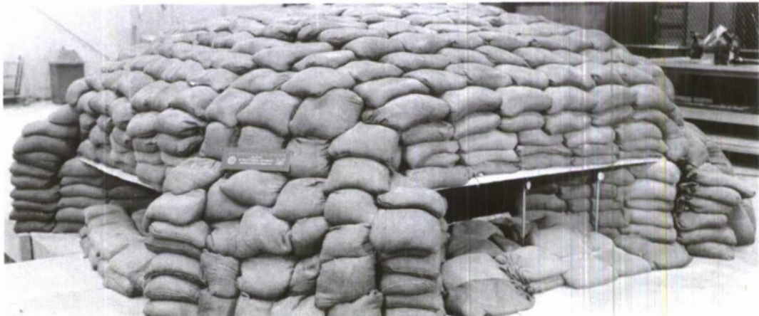
f. Six layers of sandbags
