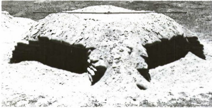
a. Crater formed by detonation of 10-pound charge above MICS crown
