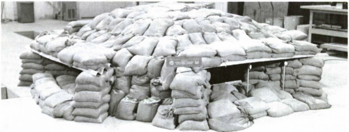
b. Two layers of sandbags
