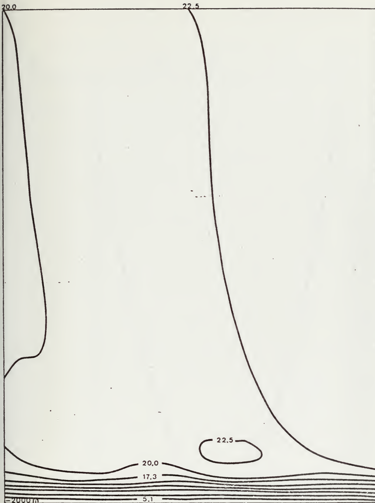
Figure 14. Numerical solution for (\partial T / \partial x)_0 > 0 and w_0 = 10 \text{ cm day}^{-1} , (\partial / \partial z)(w'T') = 0 . Temperature is in ^{\circ}\text{C} .
